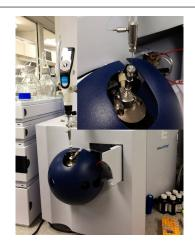
Figure 5. Direct infusion of eVol MEPS into ESI source.
