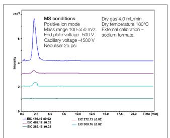
Figure 6. Extracted ion chromatogram of dilute urine processed using MEPS and infused directly into the ESI source.
