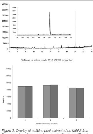
Figure 2. Overlay of caffeine peak extracted on MEPS from three operators. Inter-operator repeatability, three different operators, two independant extractions, same day same MEPS cartridge. Six injections = 4.17% RSD (auto injector repeatability on six standard injections = 2.94% RSD).
