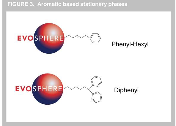
Although the Phenyl phases shown in figure 3 appear similar the addition of the branched structure in the Diphenyl phase chemistry leads to significant selectivity changes due to the extra steric interaction that occurs around the branched structure. With multiple interactions tacking place difficult to resolve compounds, such as positional isomers and metabolites, are no longer the problem they once
