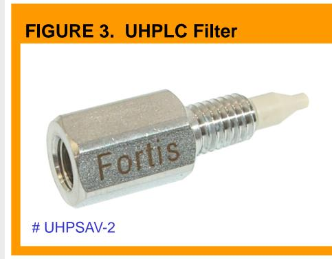
The Fortis<sup>™</sup> UHPLC Filter (figure 3) is a pre-column filter that is suitable for operation under UHPLC conditions. It contains a 0.2um porous frit and is designed to possess minimal dead volume, this ensures that it does not significantly contribute to any band broadening.
